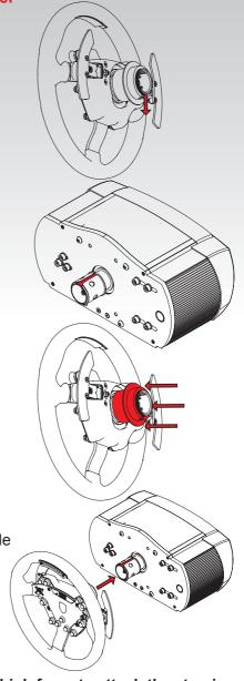
IMPORTANT: Please mind not to use high force to attach the steering wheel to avoid damages! It is possible to attach the steering wheel on the last 8 mm you need a little force because of the O-ring which avoids shaking steering wheels.
